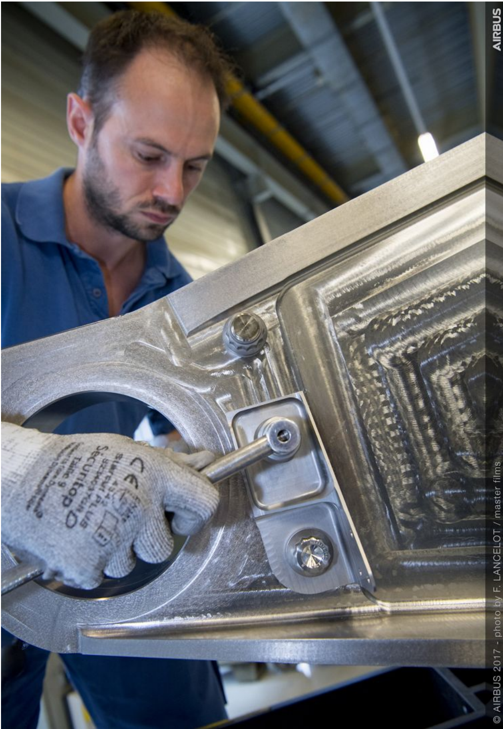
3D printed bracket installed on A350 XWB pylon
