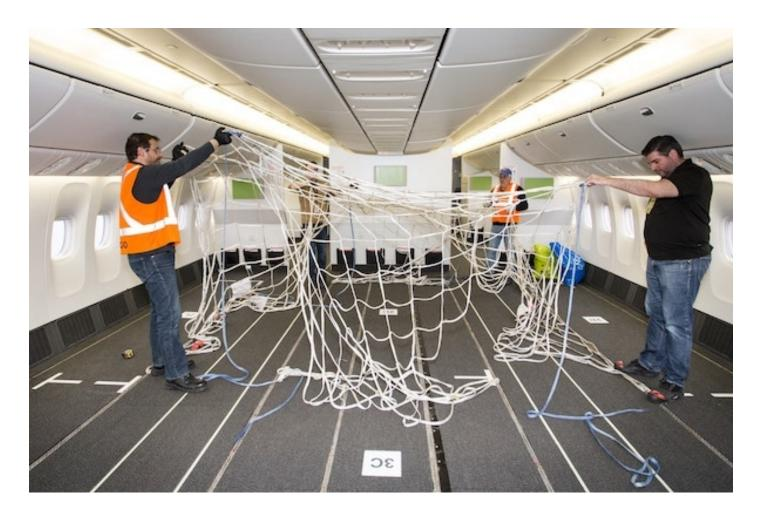
Air Canada is reconfiguring the cabins of three of its Boeing 777-300ER aircraft to give them additional cargo capacity. The first aircraft conversion is complete and is now in service, with the second and third aircraft to be completed shortly.
