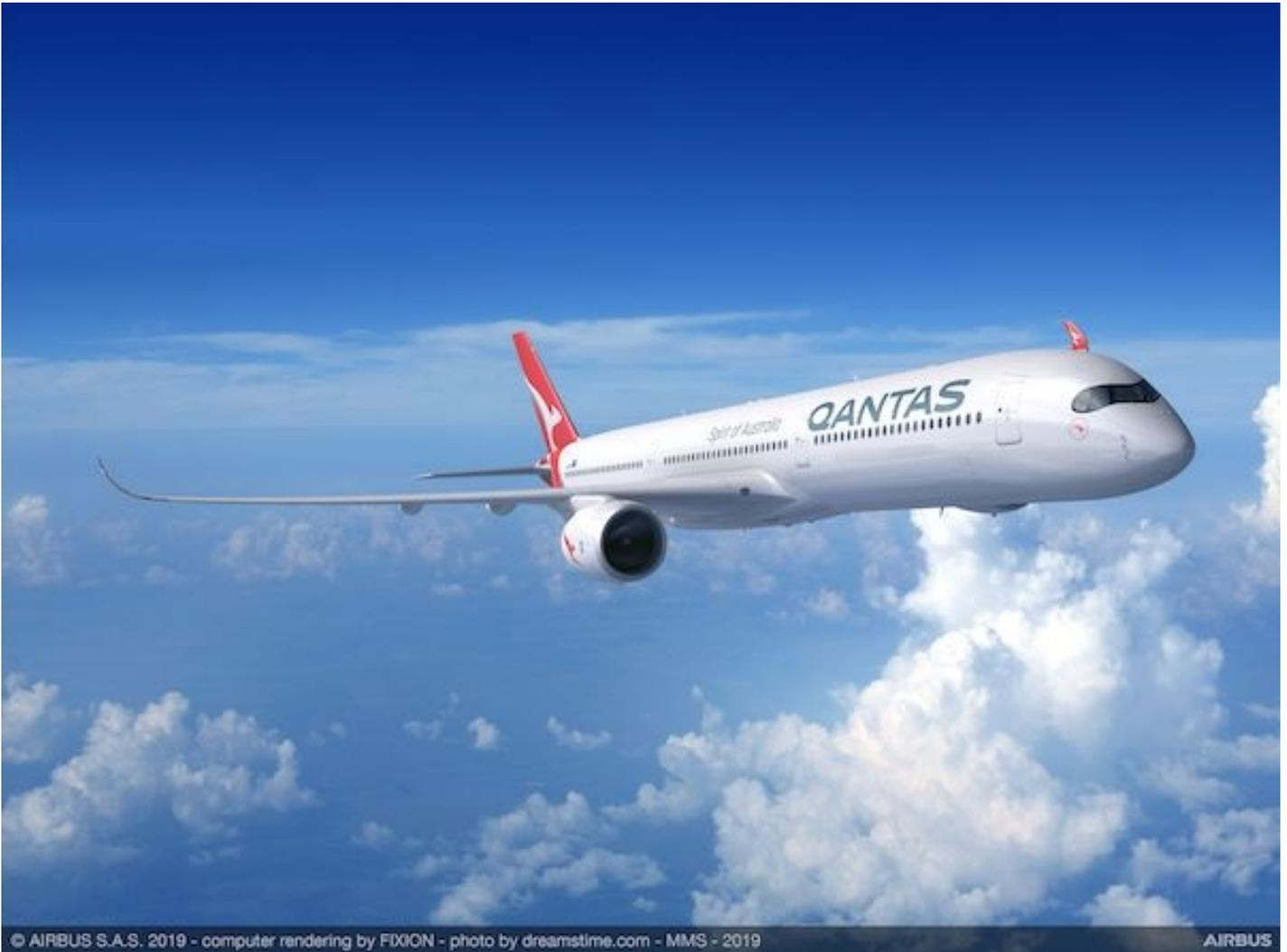
After detailed evaluation of the Boeing 777X and Airbus A350, Qantas has selected the A350-1000 as the preferred aircraft if Sunrise proceeds. This aircraft uses the Rolls Royce Trent XWB engine, which has a strong reliability record after being in service with airlines for more than two years. Airbus will add an additional fuel tank and slightly increase the maximum takeoff weight to deliver the performance required for Sunrise routes.
