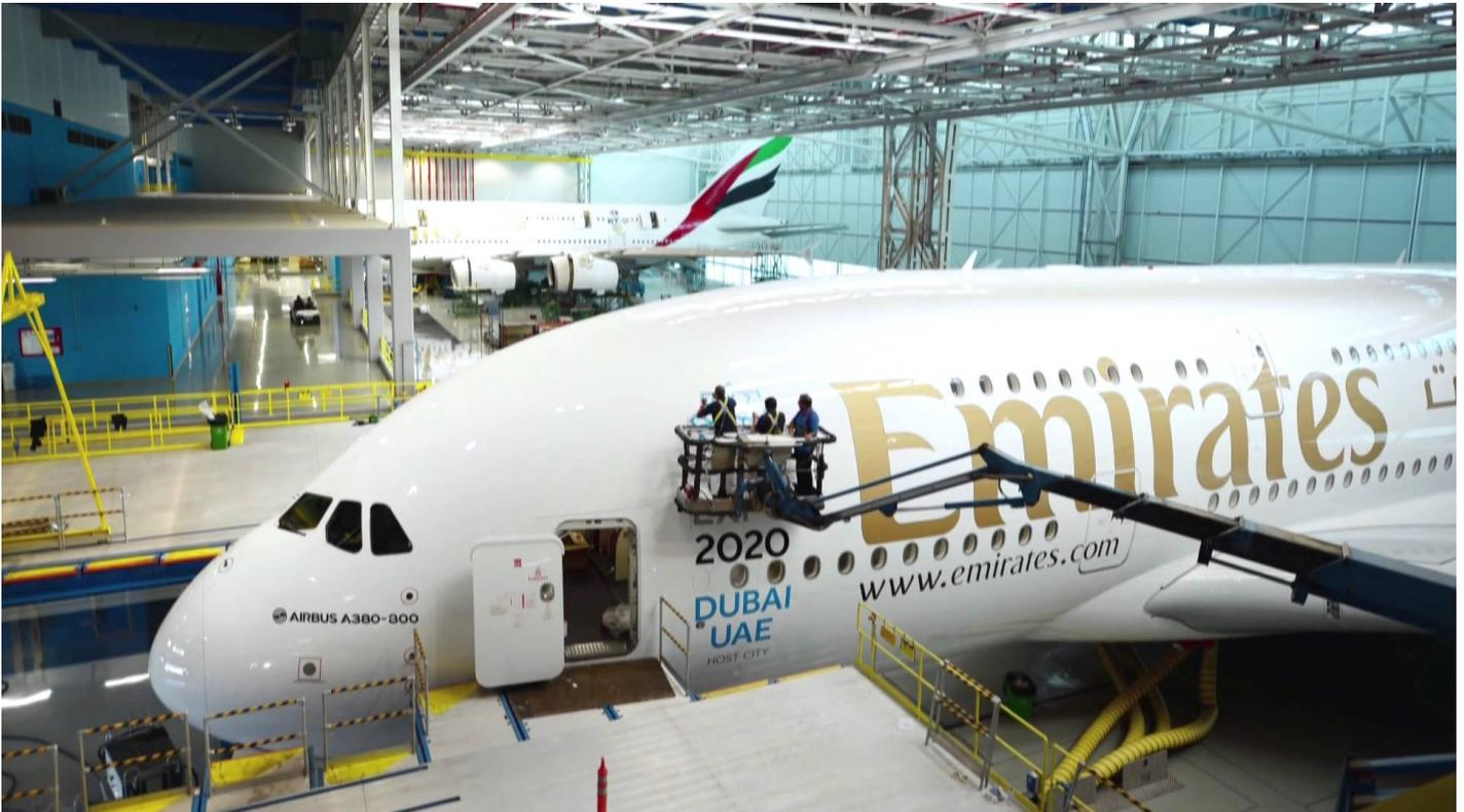
**The Emirates Aircraft Appearance Centre, the world's largest aircraft painting facility owned by an airline, has completely stripped and repainted 33 aircraft last year, or 13% of its fleet.**
