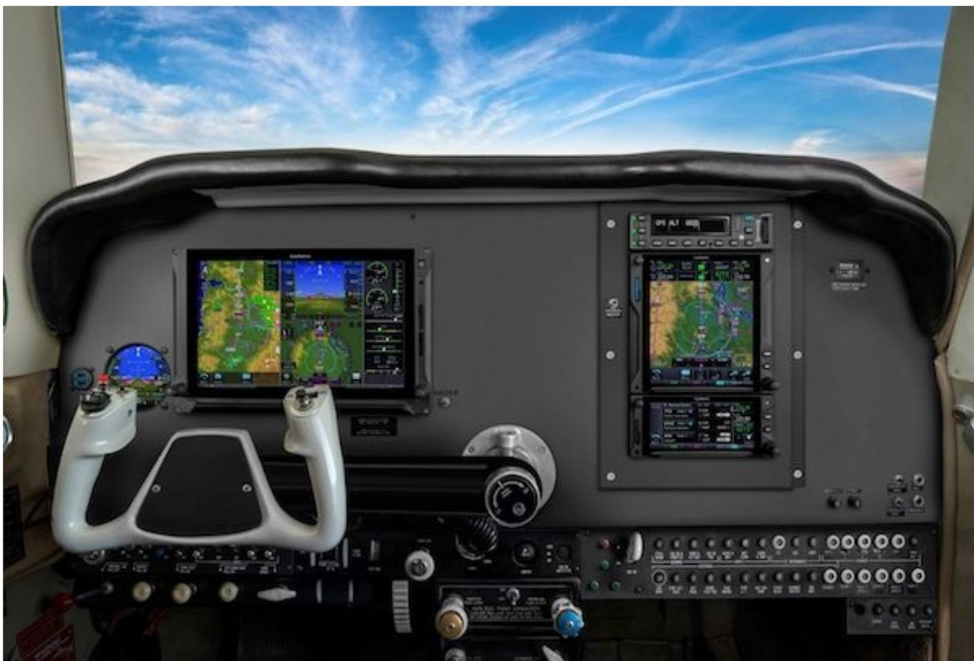
**Garmin announced new features for the GTN Xi Series of navigators including a Glide Range Ring that helps safety-minded pilots visualize the estimated area an aircraft could reach in the case engine power is lost<sup>1</sup>. Other new features include the ability to remotely control the radios of another GTN Xi when dual GTN Xi units are installed in an aircraft, quicker page navigation with the addition of customizable dual concentric knob functions, and more.**
