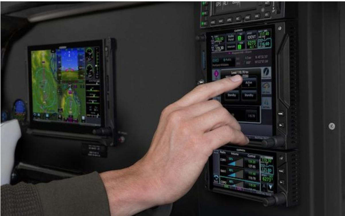
Remote radio control allows pilots to tune and radio frequencies from a single GTN Xi navigator
