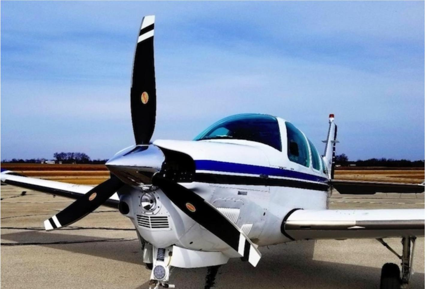
**Hartzell's new Navigator, a three-blade advanced structural composite scimitar propeller, is now approved for thousands of Beechcraft Bonanza single-engine airplanes.**
