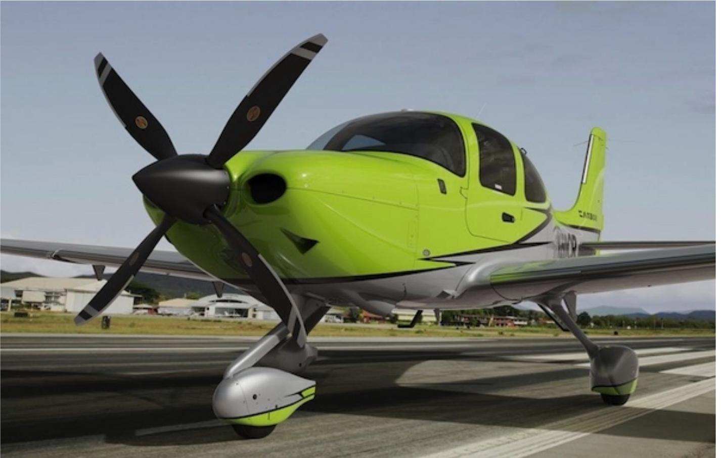
**Cirrus SR22 and SR22T pilots can now add Hartzell Propeller's four-blade structural composite carbon fiber propeller, called the Odyssey, to their airplanes for \$35,000. The new propeller has been available as an STC option for new aircraft from the factory since earlier this year.**
