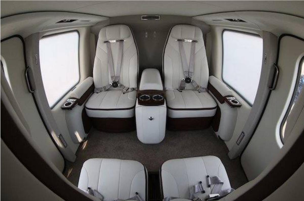
The design specifics of the convertible Mi-171A2 make it possible to convert the helicopter's cargo compartment into a passenger cabin at the operator's facilities within one hour. Mi-171A2 can transport up to 20 passengers on energy-absorbing seats and up to 5 tons of cargo on an external sling.
