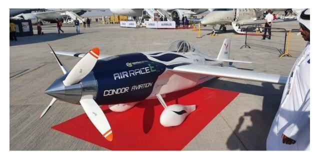
Team Condor leader Martyn Wiseman and his crew have spent the past months converting White Lightning into a fully-electric racing machine, utilising a Contra Electric twin motor and contrarotating propeller powertrain.
