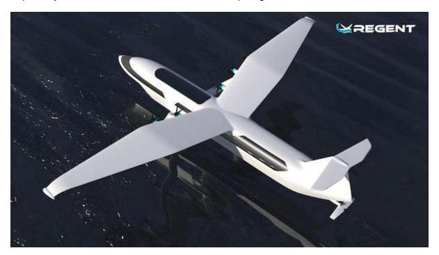
REGENT's mission is to drastically reduce the cost and headache of moving people and goods between coastal cities. Our vehicle, called a seaglider, is an all-electric, wing-in-ground-effect craft that operates within a wingspan of the water's surface and couples the speed of an airplane with the operating cost of a boat. Built to the same safety standards as all modern aircraft and watercraft, sour setting battery here anology and
