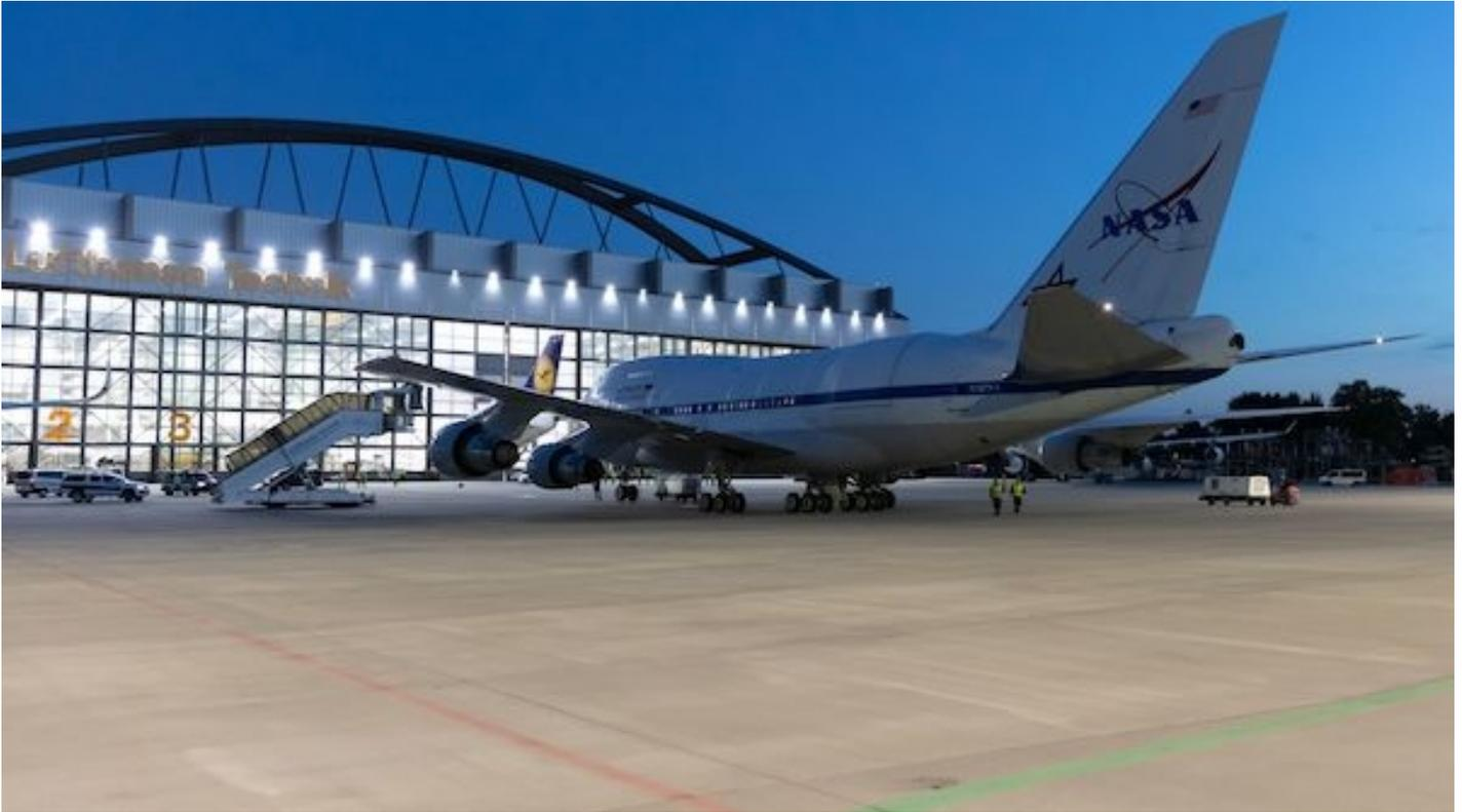
**Stratospheric Observatory for Infrared Astronomy, a modified Boeing 747SP, is due for another "pit stop": For a routine check at Lufthansa Technik, the flying observatory of the US space agency NASA and the German Aerospace Center landed at Hamburg Airport on 30 September 2020. During this layover, which is equivalent to a C-check taking place approximately every three years, the Boeing 747SP is put through its paces.**
