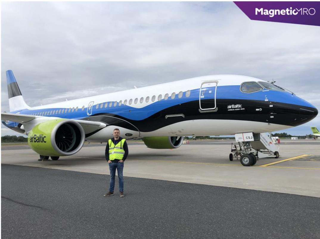
To create this artwork, 15 professional painters worked for 1 000 hours. In total, 250 litres of primer, paint and lacquer were used to cover the aircraft, which constitutes the layer of 120 microns or 0.12 mm.
