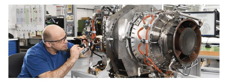
For the first time, RUAG Aviation has overhauled a Pratt & Whitney Canada PW206 engine. The maintenance of the engine that is used in the Airbus H135 and H135M helicopters was carried out in the engine maintenance shop in Stans. The fact that the PW206 engines can now be maintained in-house at RUAG Aviation will help to increase the availability of the Swiss Air Force's helicopter fleet.
