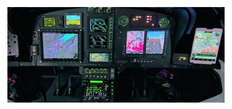
RUAG has designed, developed and integrated a Supplemental Type Certificate (STC) featuring Night Vision Imaging Systems (NVIS) for the new Airbus Helicopters, Inc. H125. RUAG realized the STC on behalf of customers Swiss Federal Office of Civil Aviation (FOCA) and Swiss Transportation Safety Investigation Board (STSB).
