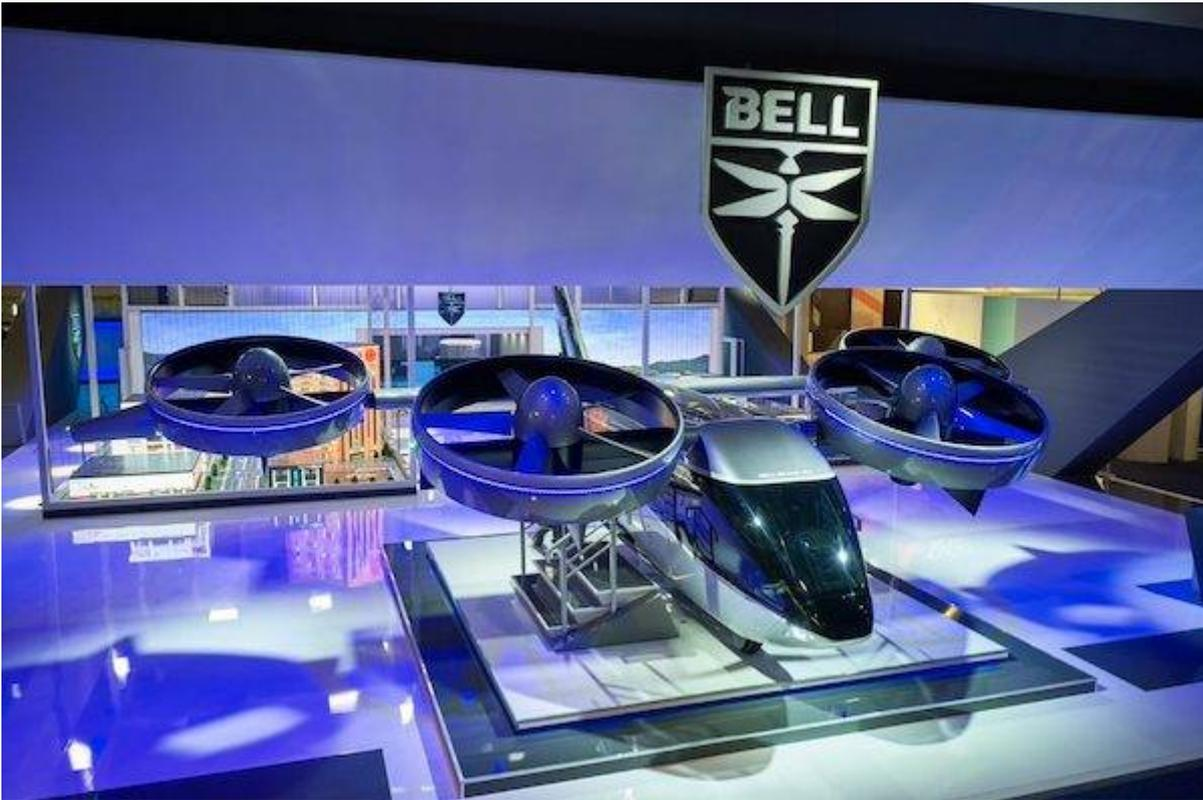
BAC was recently contracted by Bell to build ducts for their Nexus 4EX air taxi mockup, which was on display at the Consumer Electronics Show in Vegas last month. BAC engineered and manufactured the four complete duct assemblies including the outer duct rings, center cowling, vanes, control surfaces, and spinners and propellers. They were able to create a high temperature, dimensionally stable, and cost-effective tooling solution to manufacture these parts for the full-size mockup.
