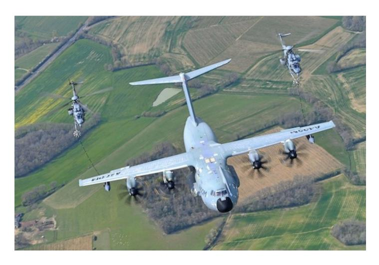
The Airbus A400M new generation airlifter has successfully conducted a major helicopter air-to-air refuelling certification campaign, completing the majority of its development and certification objectives. Airbus Defence and Space aims to achieve full helicopter air-to-air refuelling certification later this year with the conclusion of all mandatory night operation trials.
