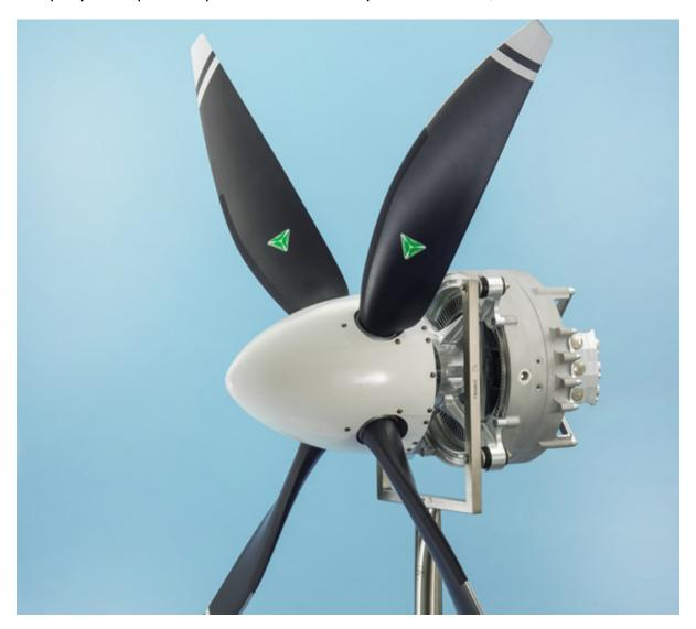
Siemens researchers have developed a new type of electric motor that, with a weight of just 50 kilograms, delivers a continuous output of about 260 kilowatts – five times more than comparable drive systems.
