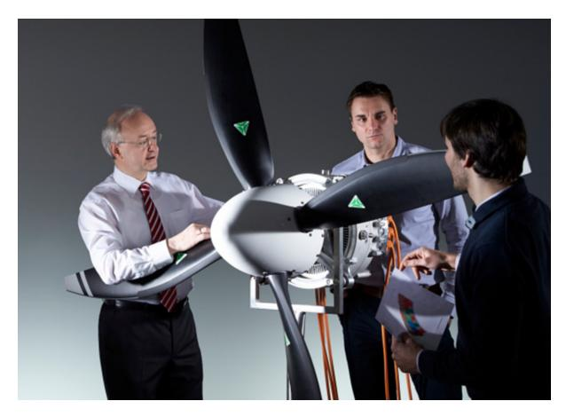
High-power: The new electric motor has a power/weight ratio of a five kilowatts per kilogram.
