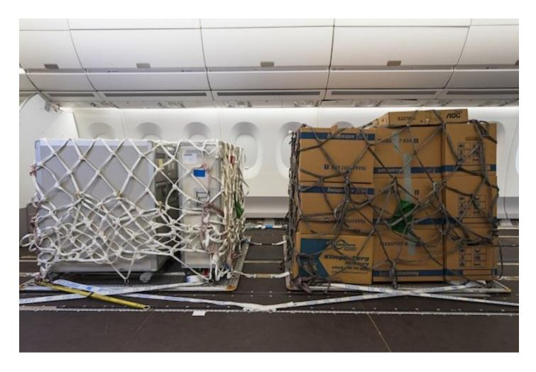
Airbus is developing a modification for A330 and A350 family aircraft which will enable airlines to install freight pallets directly onto the cabin floor seat tracks, after removal of the economy-class seats.
