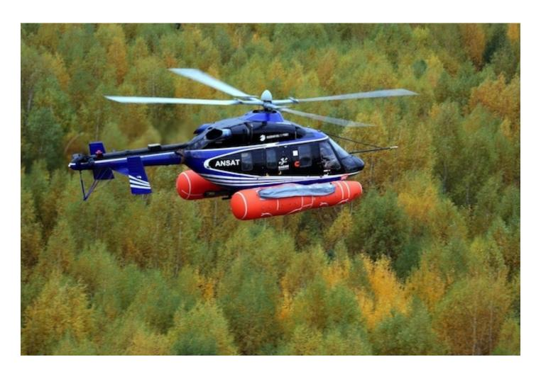
The Federal Air Transport Agency - Rosaviatsiya, certified the installation of the Emergency Floatation System on Ansat helicopter. It is designed for emergency water landing and is used to save lives of the crew and passengers. Rosaviatsiya also issued Kazan Helicopters of Russian Helicopters holding company the approval for the main change: the reduction in airworthiness limitations of several main parts of Ansat.
