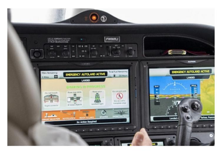
Daher HomeSafe is certified on its TBM 940, authorizing the availability of this emergency autoland system that would automatically bring the aircraft to a runway touchdown if the pilot becomes incapacitated. HomeSafe received its approval from both the European Aviation Safety Authority (EASA) and U.S. Federal Aviation Administration (FAA) airworthiness authorities.
