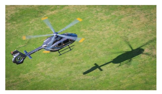
Visible on the Airbus booth at the show, this latest upgrade brings a new, innovative fivebladed rotor to the multi-mission H145, increasing the useful load of the helicopter by 150 kg while delivering new levels of comfort, simplicity and connectivity.
