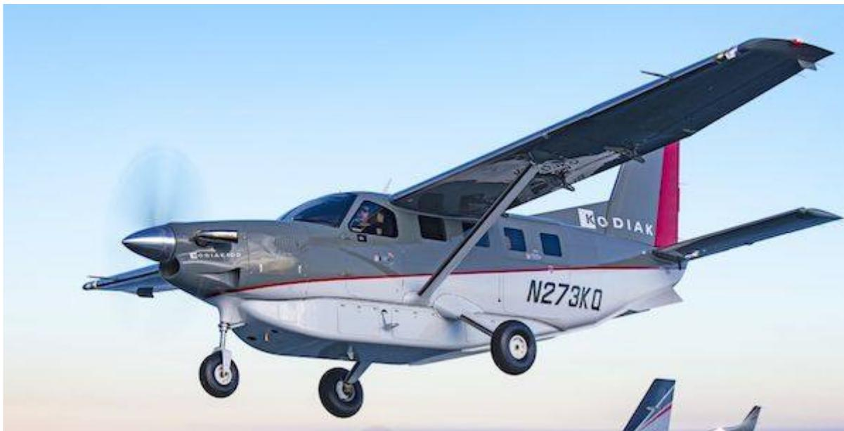
The Kodiak 100 Series II is an unpressurized 10-seat airplane equipped with Garmin's G1000 NXi avionics, capable of operating on uneven and ultra-short runways, or on water in the amphibious version. Its unique combination of robust construction and remarkable 3,535 lbs (1,603 kg) maximum payload capability has resulted in many additional applications for the Kodiak, including special missions, medevac, as a skydiving platform and more.
