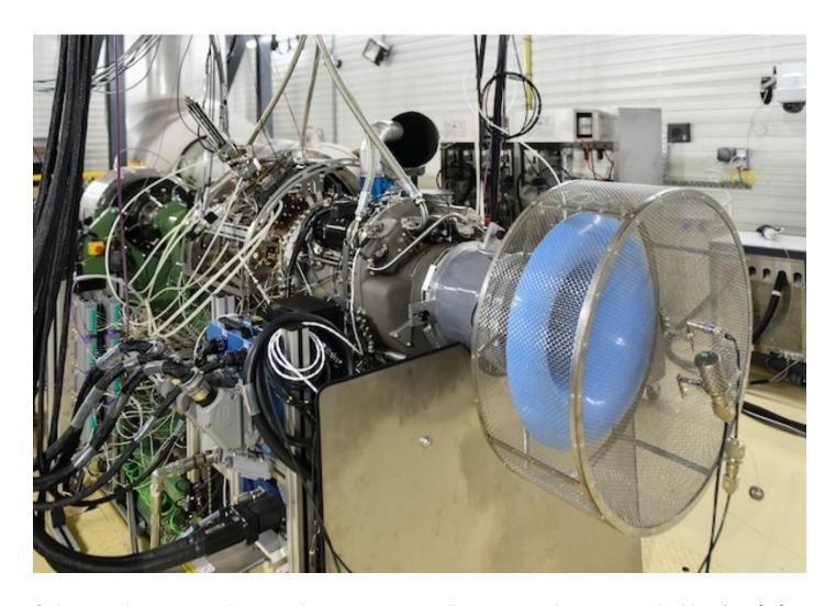
Safran Helicopter Engines performed a world first test at its Bordes facility (Pyrénées-Atlantiques, France); a helicopter engine run on 100 percent sustainable aviation fuel (SAF). During the test, a Makila 2 ran on a biofuel produced by TotalEnergies from residues and waste from the circular economy, specifically used cooking oil.
