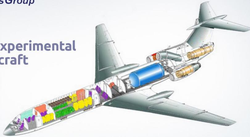
Tu-155 was the first experimental aircraft in the world operating on hydrogen.
