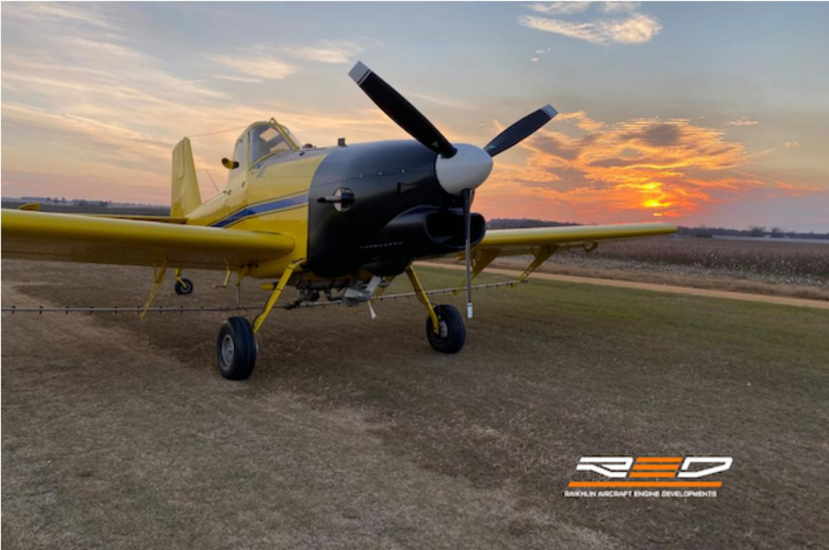
The cowling section of the AT-301 was purposefully redesigned to accommodate the RED A03 engine and provide a more aerodynamic shape. To avoid a significant weight increase, the cowling was manufactured from lightweight carbon fibre and is custom built to include cooling, sufficient air intake, and service access points.
