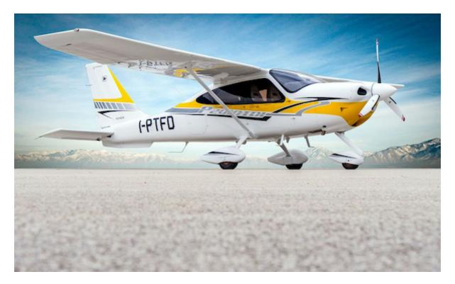
The P2010 TDI role is to fill a gap in customer choices, as they can now order the "Twenty-Ten" with three different powerplants, and three different fuel capabilities: automotive unleaded (approved on 180hp version), Avgas on the most powerful 215hp variant and, from now on, Jet/diesel.
