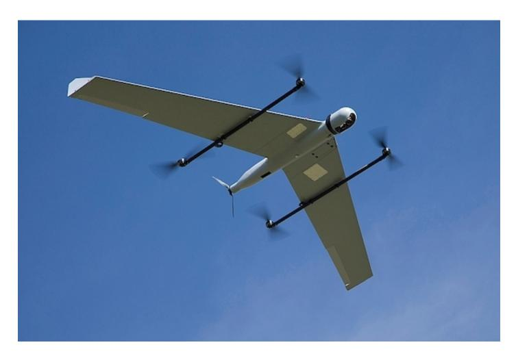
ZALA Aero has developed a new multipurpose VTOL unmanned aerial vehicle ZALA 421-16EV. The new unmanned VTOL ZALA 421-16EV HD features a unique adaptive system for using the aerodynamic properties of UAV in all flight modes. The new unmanned system combines the latest scientific and technical developments of the company - it broadcasts the video stream in HD quality (1280\*720), which allows the ground station operator to examine the streaming video in the detail.
