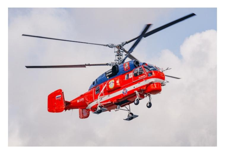
Russian Helicopters will present a modernized Ka-32A11M fire-fighting helicopter at the MAKS-2021 International Aviation and Space Salon, held in Zhukovsky near Moscow in July. Ka-32 modernization program includes a glass cockpit with an avionics system, more powerful VK-2500PS-02 engines and a new fire extinguishing system.
