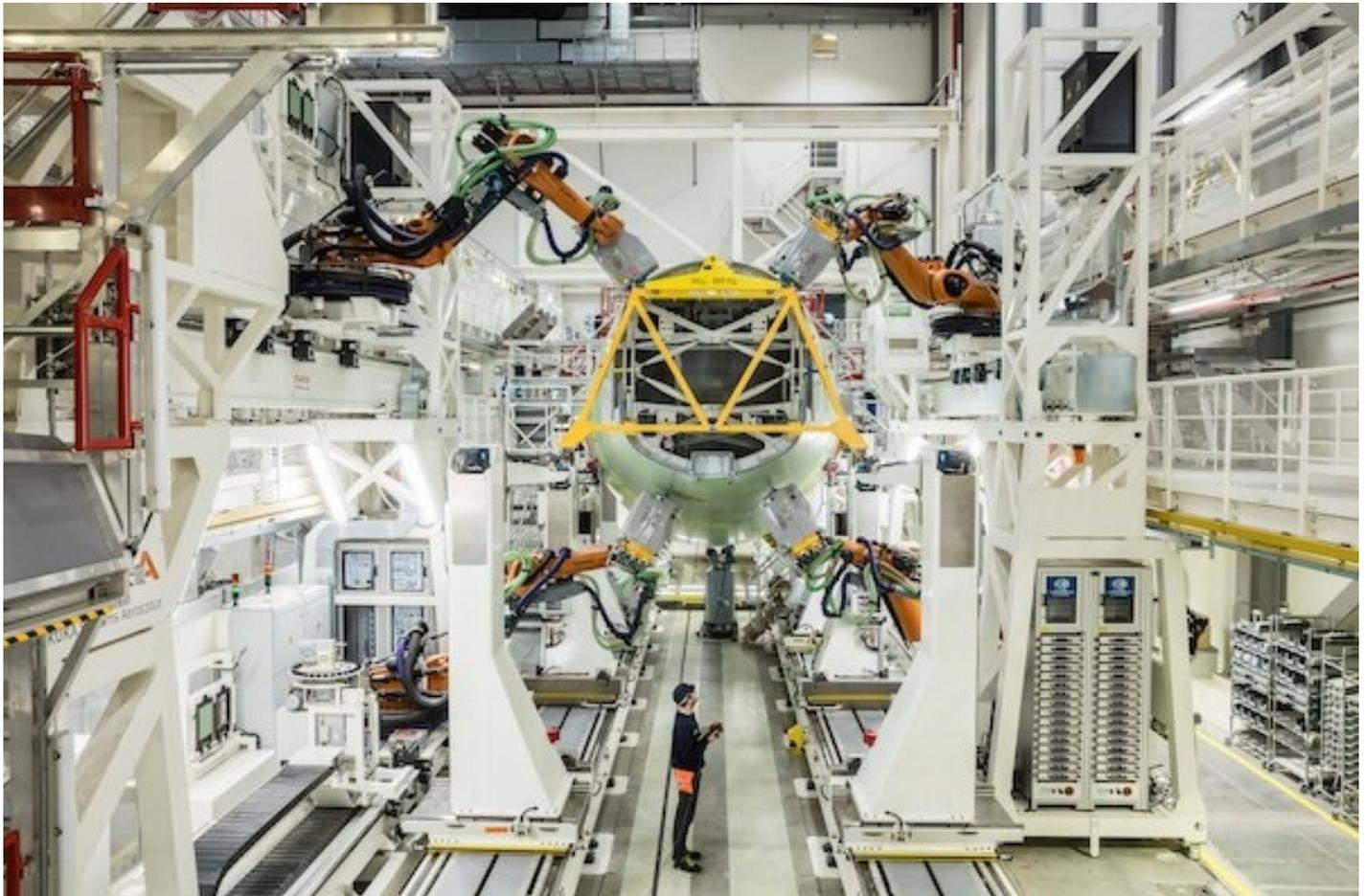
**A highly automated fuselage structure assembly line for A320 Family aircraft in Hamburg is inaugurated!**
