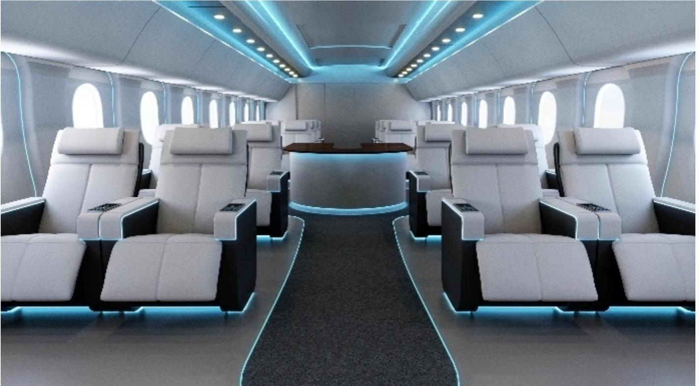
**Astronics Corporation introduced new Nuancia RGBW Strip Lights to provide flexible illumination options for aircraft seats and cabins. With this system, aircraft manufacturers and airlines can program mood-lighting systems to accommodate more than 16 million colors, create preset color scenarios, and present color changes.**
