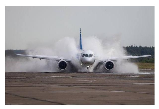
In the process of testing the possibility of safe movement on a wet runway in a wide range of speeds without any failure of marching and auxiliary power plants, as well as other systems and equipment of the aircraft were confirmed.
