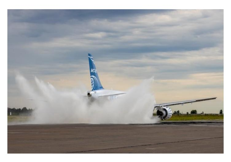
Irkut Corporation summarized the preliminary results of MC-21-300 aircraft ground testing, which confirmed the possibility of operating the aircraft in presence of water on runway. During the period from 16 to 22 July 2020, the MC-21-300 aircraft performed 29 runs and 3 taxing on water at speeds from 10 to 150 knots (1 knots = 1.852 km/hour) at various configurations of mechanization and power plant modes, including the use of engines thrust reversal.
