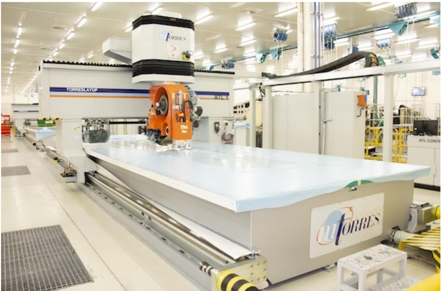
**Strata has deployed two of the latest generation MTorres Automatic Tape Laying machines to support its Airbus A350-900 manufacturing capabilities. The AI Ain based manufacturer has gained First Part Qualification and First Article Inspection design and quality verifications for the use of the computer-controlled robotic ATL machines that will automate Strata's production of the Inboard Flap components.**
