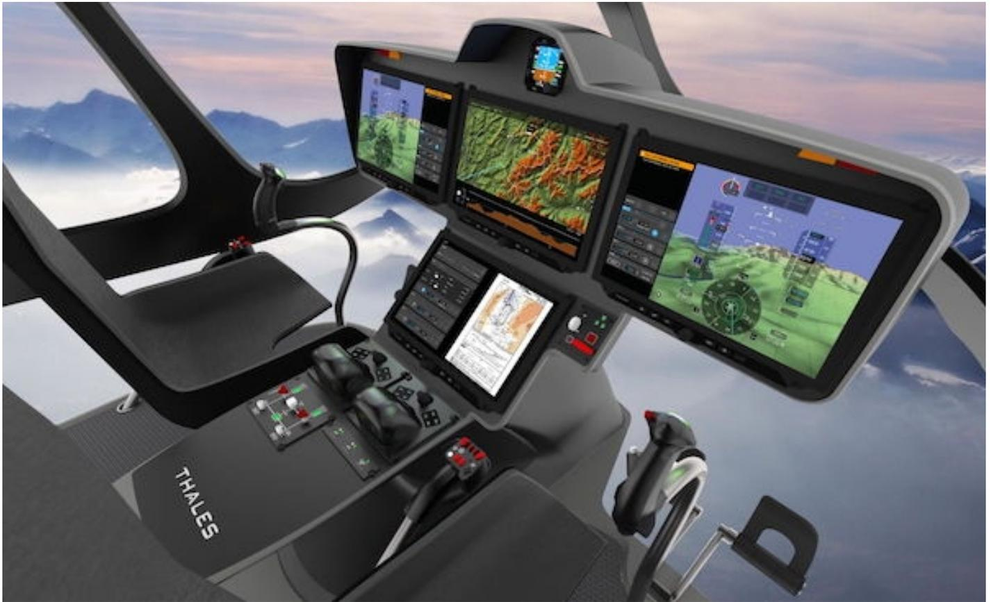
The FlytX avionics suite will equip the future H160M Guépard, the military version of the H160 from Airbus Helicopters. FlytX is based on the Avionics 2020 concept unveiled at the 2013 Paris Air Show and comprises an intuitive touchscreen interface designed by pilots for pilots.
